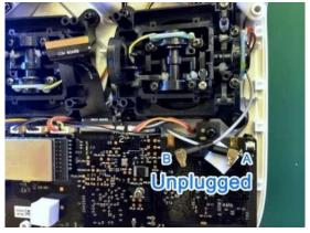
2. Snip the plastic flange then pull out Cable B.
