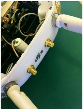
Step 4: - Route the new cables and plug under the board
