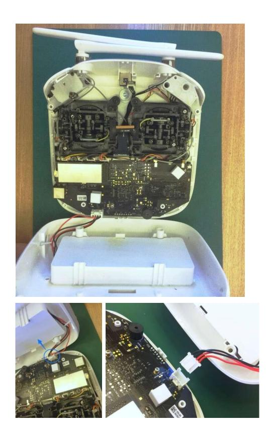
Step 2: - Unplug and pull out the original cables (A&B)
